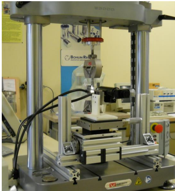
Figure III- 1: Machine de fatigue Instron E3000
