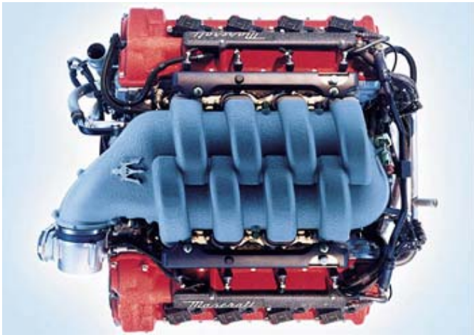
Figure 3: View of the V8 engine, showing the intake plenum.
